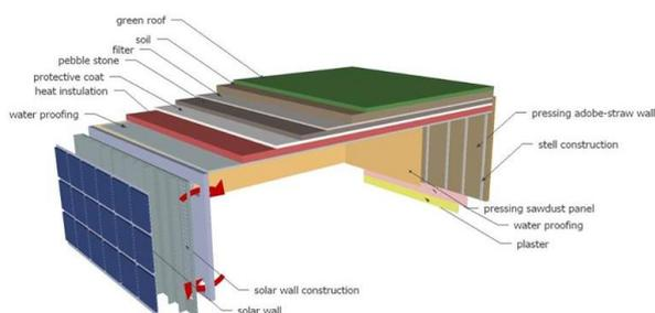
In addition, the use of Solarwall system on the south frontage of the houses is considered appropriate. This system has an air-heating system functioning with sun. Solar energy is used to heat and air-condition the internal
